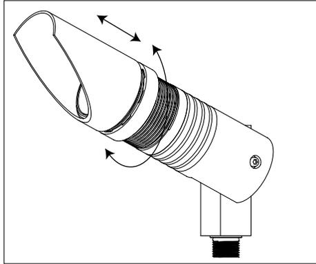
1. Rotate the locking ring clockwise to move to the desired position.
