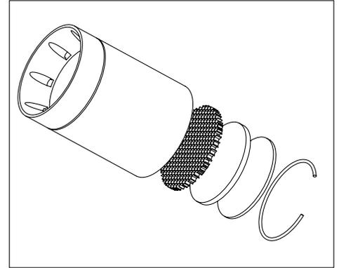
1. Rotate hood counter clockwise and remove it from body.
