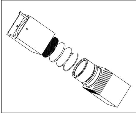
1. Use the 9/64" hex key to loosen the hood locking screw(8-32UNC hex cap screw) on the top of the hood and remove the hood from fixture body.
