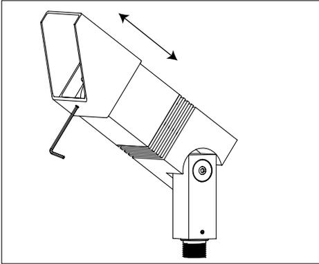
1. Use the 5/64" hex key to loosen the screw(8-32UNC set screw) on the bottom of the glare shield. Move the glare shield to the desired position, and tighten the screw (  $\Delta$  do not overtighten).
