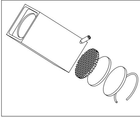
1. Use the 5/64" hex key to loosen the hood locking screw(8-32UNC set screw) on the side of the hood and remove the hood from fixture body.
